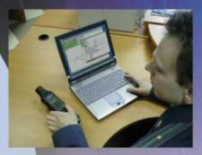
The radionuclide spectra libraries being used for identification can be selected and the instrument can be applied for resolving specific tasks
